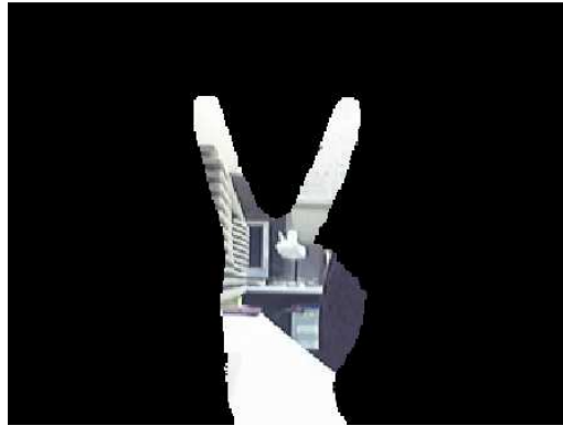
Figure 4.3: Template to teach a user how to hold his or her hand in order to be recognized by the system
