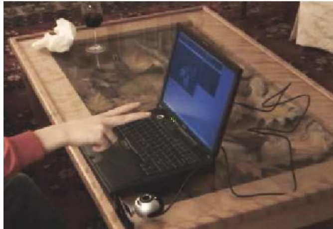
Figure 1.2: The Finger Counter . The webcam (on the table) points upward at the hand.
